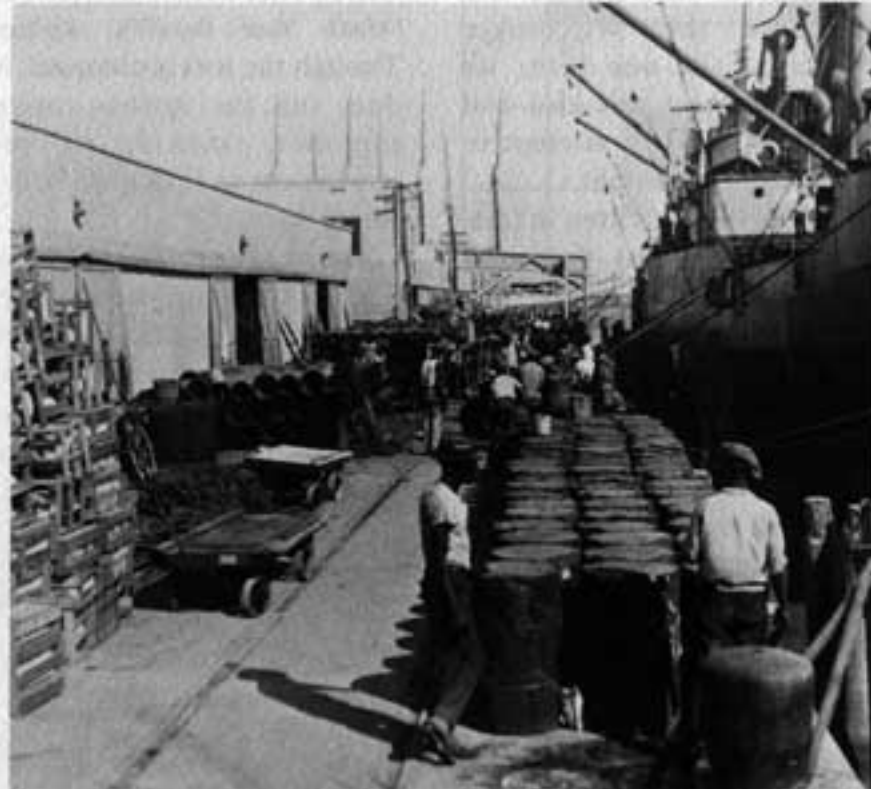
Stevedores prepare to load cargo on this ship docked in Miami. Cargo was moved by hand truck to the wharf and stacked on pallets to facilitate its transfer to the ship.
