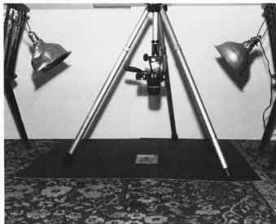
Reverse tripod's center column, spring clip two floods for even lighting of old photograph.
